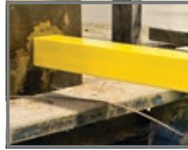
Now, it is time to turn up the heat. With the resin base now attached, the product enters a hot, steel-forming die. This hot die is pivotal to the pultrusion process as it creates the hard shape of the material.
