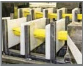
The material spools and reinforcements are threaded into a machine known as a tension roller. The roller will help to shape the pultrusions into what will soon become the finished product
