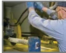
The cured profile is now advanced along a pull mechanism. The final step of the process is when the profile meets the cutting saw, where it is cut into appropriate lengths. This completes the pultrusion process and a finished fiberglass reinforced polymer is the final result.
