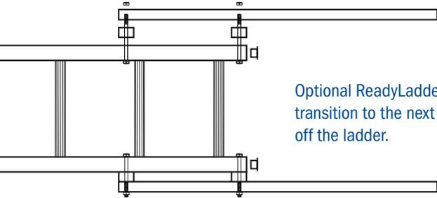
Optional ReadyLadder walk-through extensions attach to the top of the ladder to provide a safe, easy transition to the next surface. The OSHA-compliant extended sides give workers a handhold as they step off the ladder.
