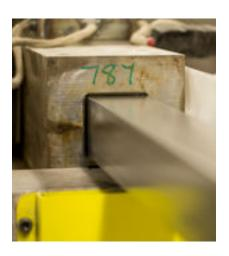
**Curing** Wet-out reinforcements are pulled through the heated pultrusion die, which begins the thermosetting process that causes the resin to "cure" or harden. By the time the part exits the die, a solid, rigid profile in the exact shape of the die cavity has been formed with all the reinforcements laminated inside.
