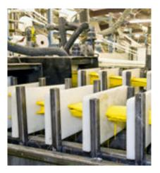
**Wet-Out** The fiberglass reinforcements are pulled through a bath of thermoset resin – typically polyester or vinylester – as well as pigments to add color, filler to enhance properties, and a catalyst to aid in curing. Resin also provides an additional form of reinforcement.
