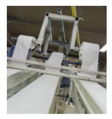
2 Surface Veil Surface veil can be added to enhance the surface appearance and provide corrosion resistance and UV protection of the final product.
