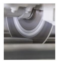
**5 Cutting** The finished product is then pulled to the cut-off saw and cut to the desired length. After cutting, it is placed in stock at one of our warehouses, sent to our state-of-the-art fabrication center for secondary processing, or crated for shipment to the customer.
