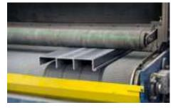
Our FRP decking is manufactured with the pultrusion process using polymer resins and fiberglass reinforcements.
