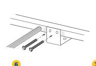
Drill holes in the ladder rails 1/16" larger than the supplied bolts, then secure the standoffs to the ladder. Torque the bolts to 60 in./lbs.; don't overtighten.
