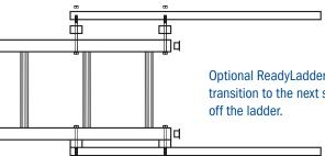
Optional ReadyLadder walk-through extensions attach to the top of the ladder to provide a safe, easy transition to the next surface. The OSHA-compliant extended sides give workers a handhold as they step off the ladder.
